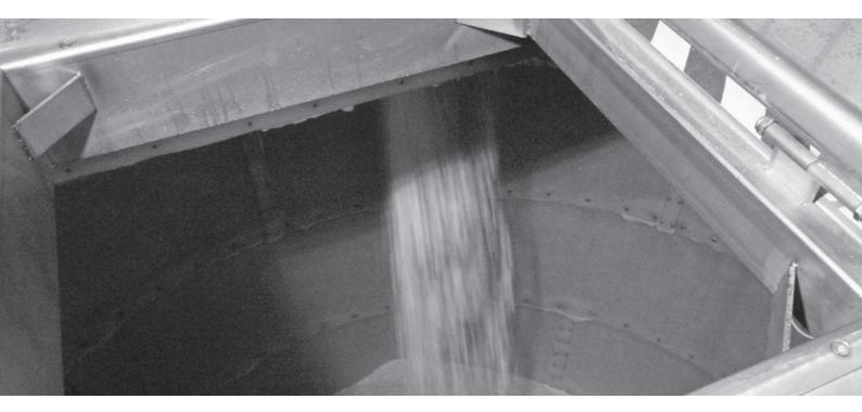
The troughed chain conveyor belongs to the continuous conveyor class. It is used for safe, covered and therefore dust-free transport over long distances. It is suitable for horizontal to vertical conveying of bulk materials such as grain, meal, and other granulated materials. Other processes such as cooling, heating or screening can be added to the transport process.
