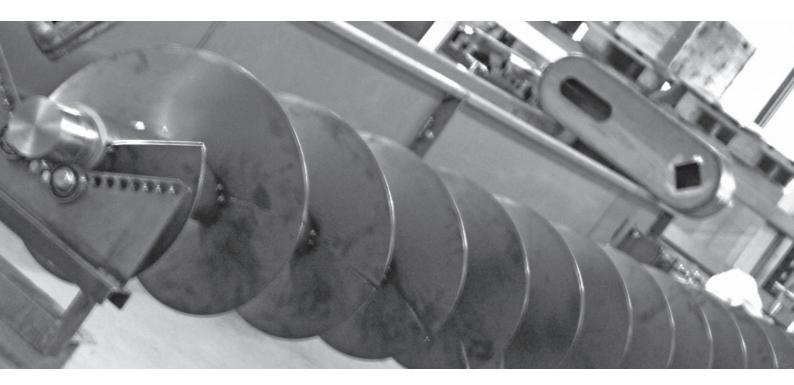
Trough screw conveyors convey the product dust-free and in a straight line over horizontal, upward and vertical distances. They are particularly suitable for granular, small, powdery, semi-wet, fibrous or bridging products such as powder, flour, cement, gravel, sand, slag or abrasive material. The large filling hopper allows a continuous filling.
