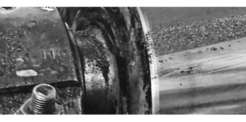
Cracking and smooth rolls wear out during use. This reduces the efficiency of the entire system when energy requirements increase. The revision of these rolls considerably improves the quality and efficiency of the mill process and is more cost-effective than a new purchase at a similar production level.
