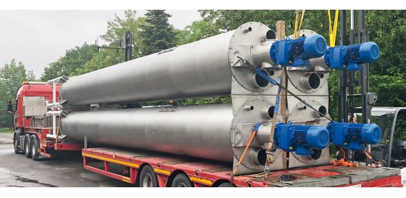
The mixing homogenizing cell TYPE MHZA from Morewa AG is suitable for mixing and homogenizing powders, flakes and granulated products. The simple process control in combination with a very powerful flow rate guarantees a continuous mixing process. The gentle and low-energy operation reduces product handling and costs considerably.
